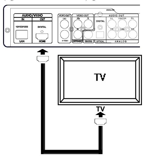
HDMI output Support HDCP (High-bandwidth Digital Content Protection)
